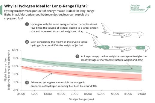
Assumptions: Aircraft design using Ala's low order aircraft design model. Cryogenic tank gravimetric efficiency ranging from 55% to 85%. Advanced hydrogen jet engine improves fuel efficiency by 10% compared to conventional jet engines.
