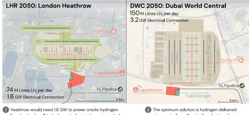
2 Heathrow would need 1.6 GW to power onsite hydrogen liquefaction for all its fuel—equivalent to the output of a large UK power station. This could be supplied via a dedicated electrical grid connection or a hydrogen-powered station. The optimum solution is hydrogen delivered via gas pipelines. On-site liquefaction plants about one hundred times larger than any existing facilities.
